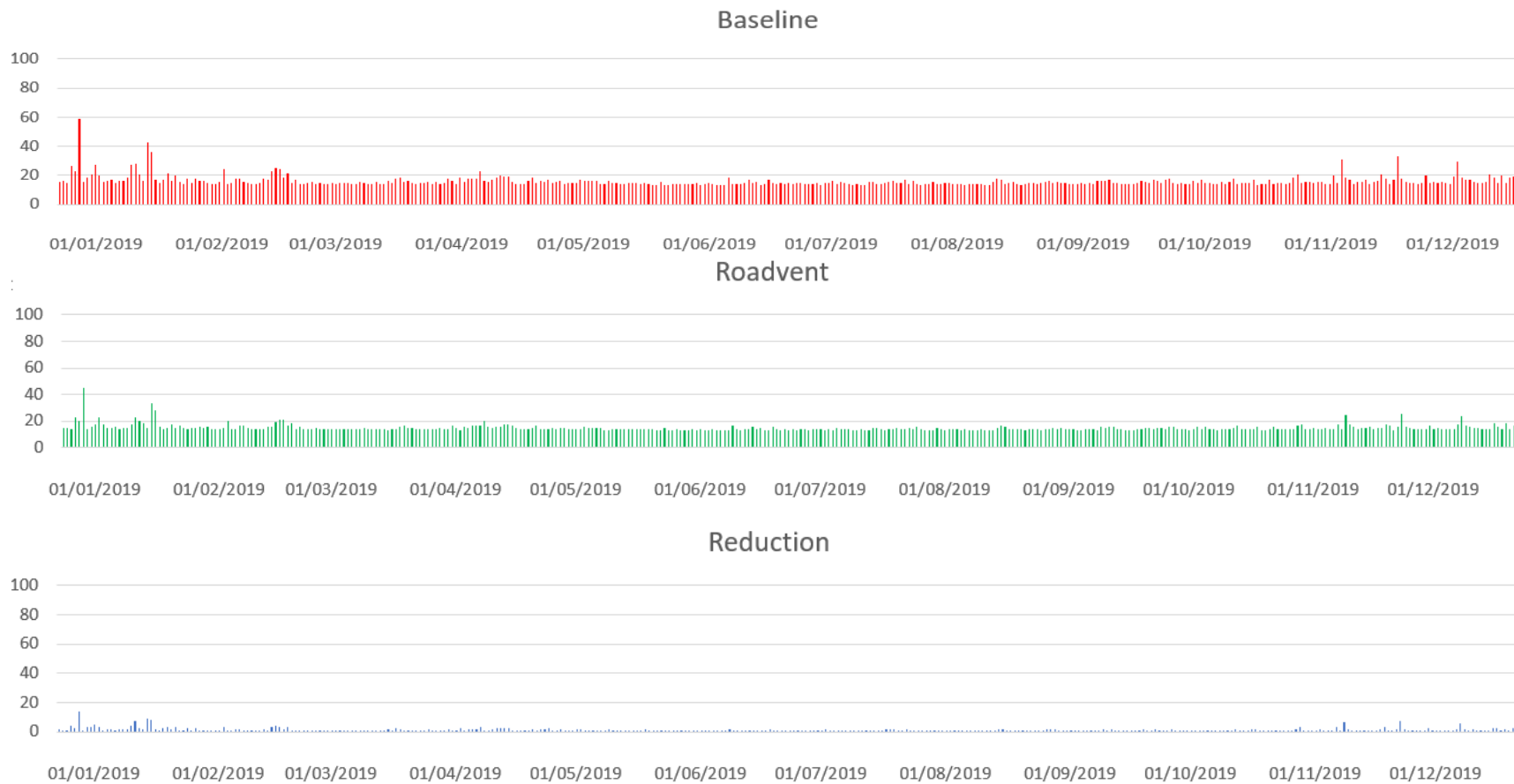
Figure 22. Modelled daily average NO 2 concentrations at baseline, with a 30m Roadvent system in RS1 and the predicted concentration reduction at the ordering. The y axis shows concentrations in \mu\text{g}/\text{m}^3 ; the x axis shows the start date for each month.
