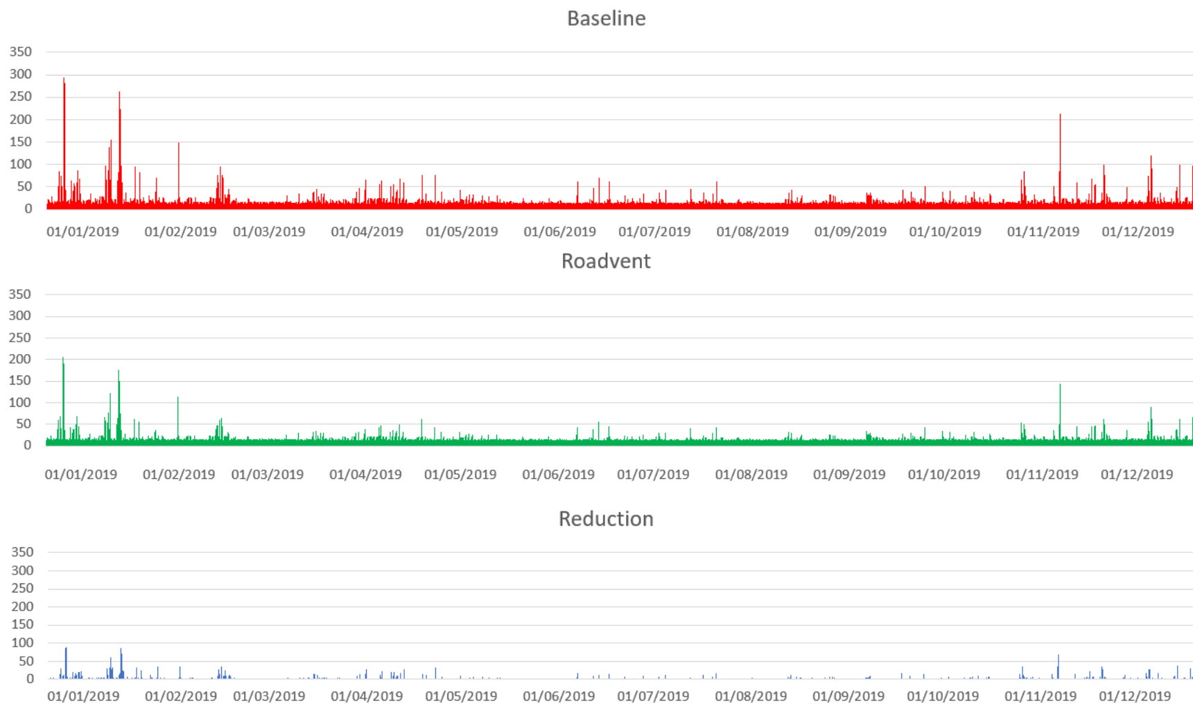
Figure 18. Modelled hourly NO 2 concentrations at baseline, with a 30m Roadvent system in RS1 and the predicted concentration reduction at the ordering point. The y axis shows concentrations in \mu\text{g}/\text{m}^3 ; the x axis shows the start date for each month.
