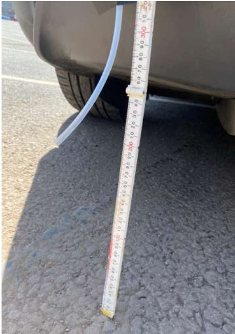
Discharge 6mm pipe exit at 180mm above road surface
