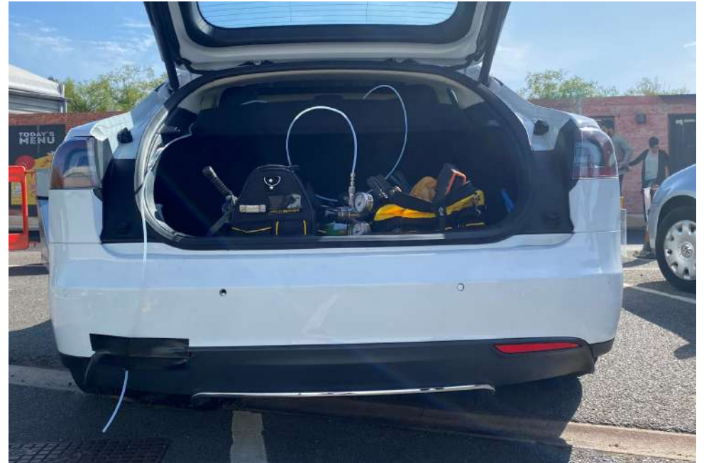
Discharge 6mm pipe exit at 180mm above road surface
